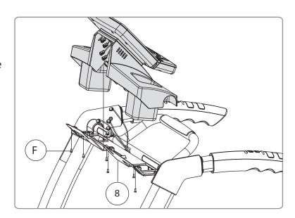
Note: Be careful to properly connect all wiring connectors with their correct corresponding wiring harness. Pay attention not to bend any pins and make sure the connectors click in place.
